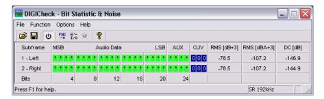
The reason for this behaviour is the noise shaping technology of the analog to digital converters. They move all noise and distortion to the in-audible higher frequency range, above 45 kHz. Therefore the noise is slightly increased in the ultrasound area. High-frequent noise has a high energy. Add the quadrupled bandwidth, and a wideband measurement will show a significant drop in SNR, while the human ear will notice absolutely no change in the audible noise floor.
