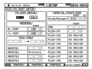
On the Remote pages 1 to 4, enter the SysEx commands described below for each channel. In the 'Layer' section, select the Remote layer 1 to 4 and select each channel with the 'select' button.
