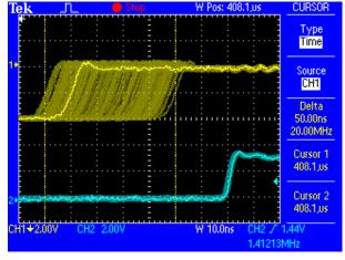
The cleaned and jitter-freed signal can be used as reference clock for any application, without any problem. The signal processed by SteadyClock is of course not only used internally, but also available at the Micstasy's word clock output. It is also used to clock the digital outputs MADI and AES/EBU.
